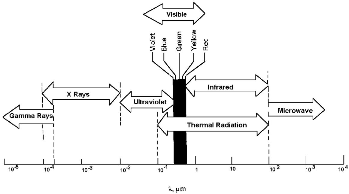
FIGURE 1. ELECTROMAGNETIC RADIATION SPECTRUM
