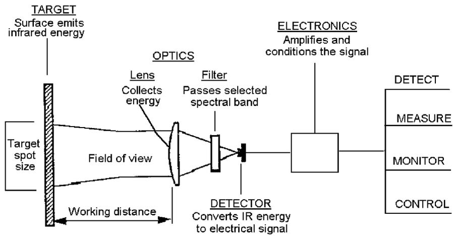
FIGURE 3. BASIC COMPONENTS OF AN INFRARED RADIATION THERMOMETER
