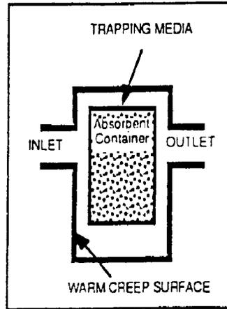
Figure 2. Absorbent Trap
