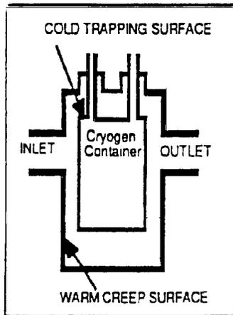
Figure 1. Condensation Trap
