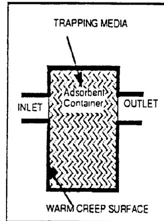
Figure 3. Adsorbent Trap
