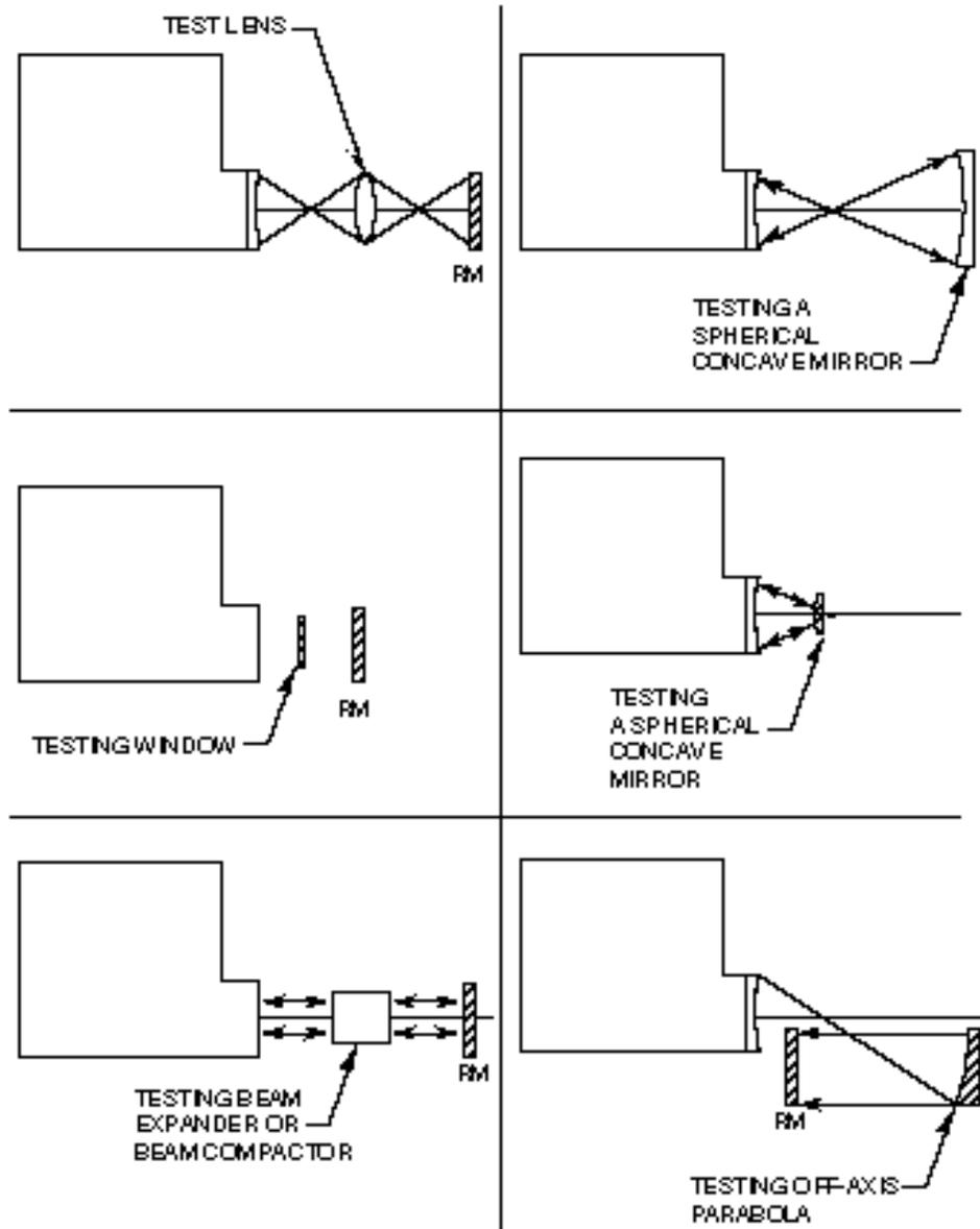
Figure 7. Configurations for testing different optical systems (from Ref. 1)
