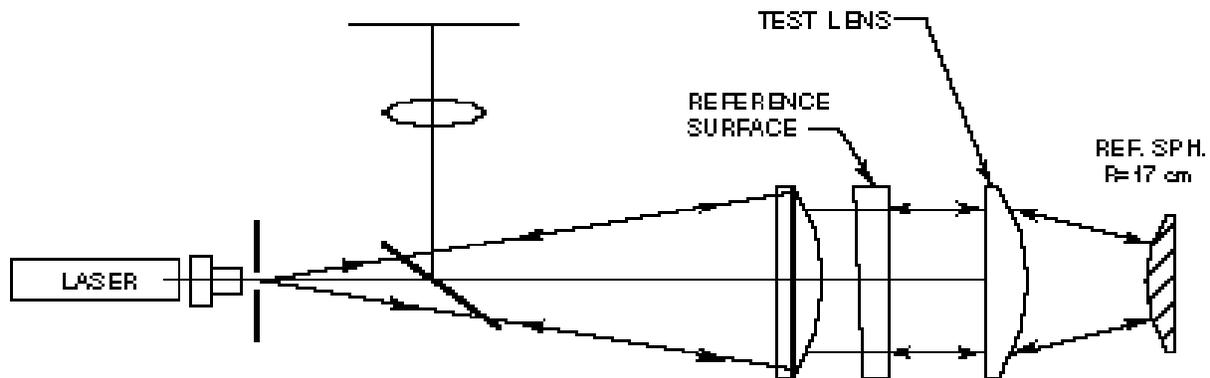
Figure 8. Test arrangement using long radius convex reference sphere to reduce retrace error
