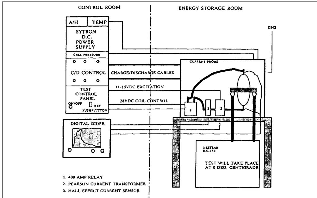
Figure 2: Ni/H<sub>2</sub> Cell Short Circuit Test Block Diagram
