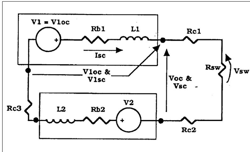
Figure 5: Dual Cell Equivalent Circuit Model
