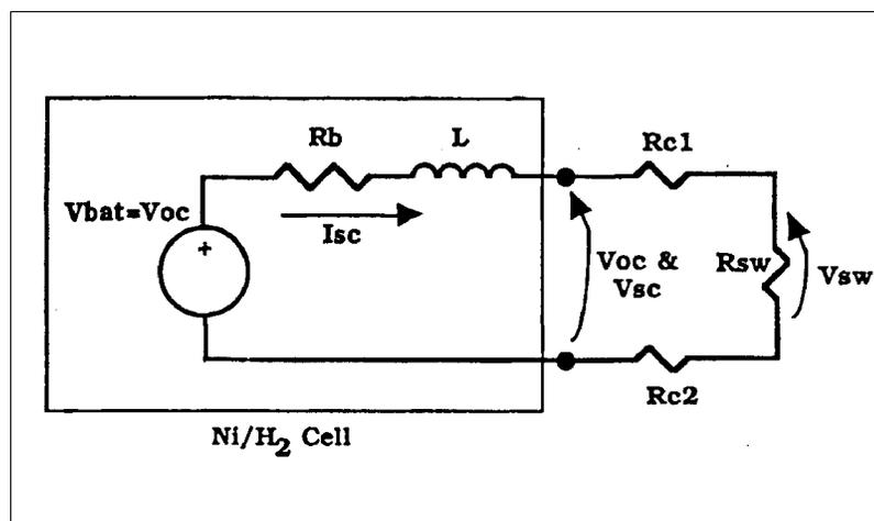
Figure 4: Single Cell Equivalent Circuit Model
