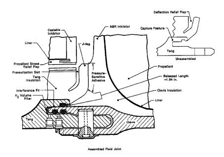
Figure 1. Cross-section of Field Joint
