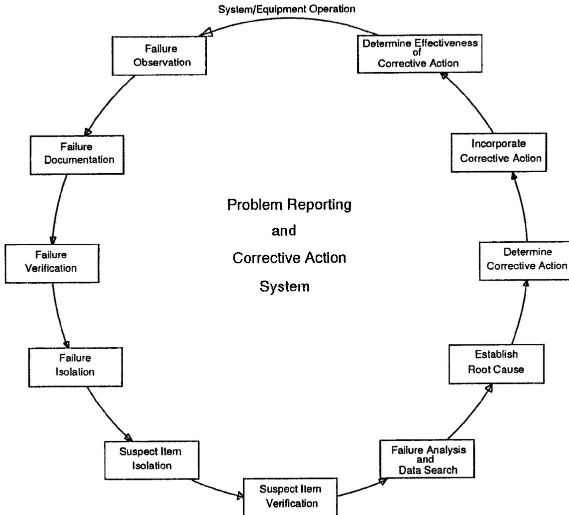
Figure 1. Closed-loop Problem Reporting and Corrective Action System
