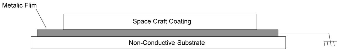
**Figure 1. Method for grounding spacecraft coating to a nonconductive substrate**
