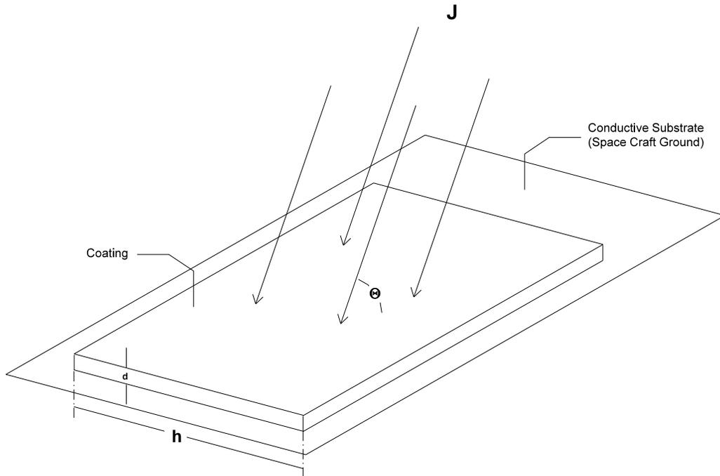
**Figure 2. Space Craft Coating on a Conductive Substrate**
