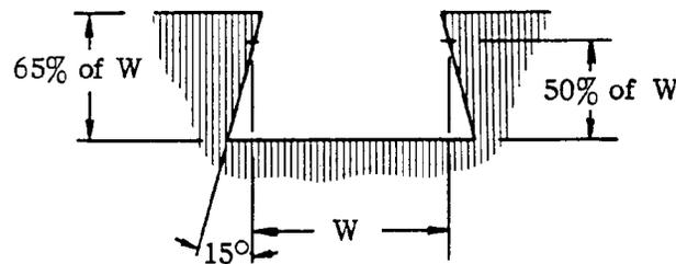
**Figure 1. O-Ring Groove Dimensions for Vertical Position**
