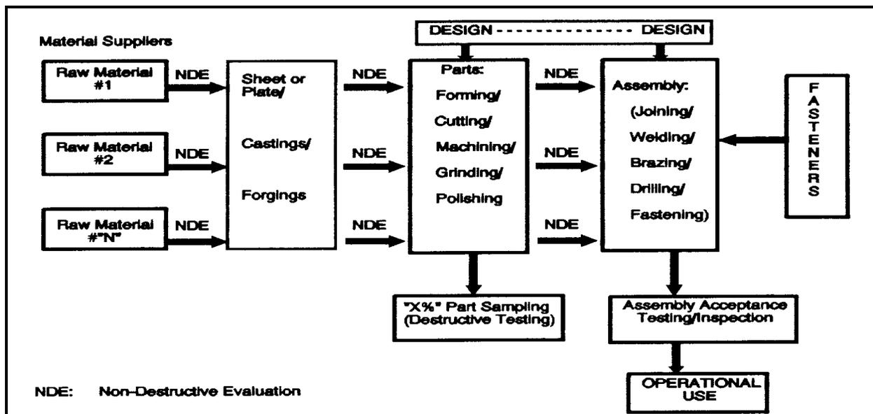
Figure 1. Conventional Metals Design, Manufacturing, and Testing
