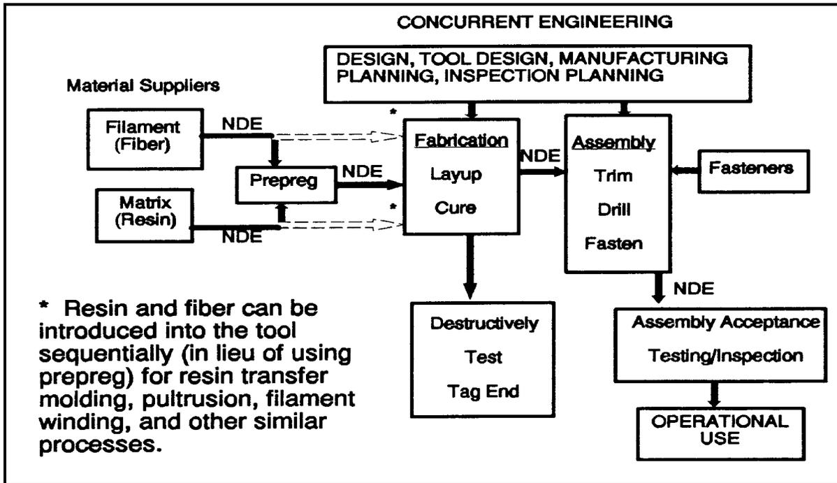
Figure 2. Structural Laminate Composites Design, Manufacturing, and Testing
